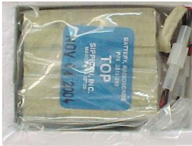
Figure N-15 – Battery in Compartment
