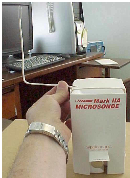
Figure N-3 – Orienting Boom
