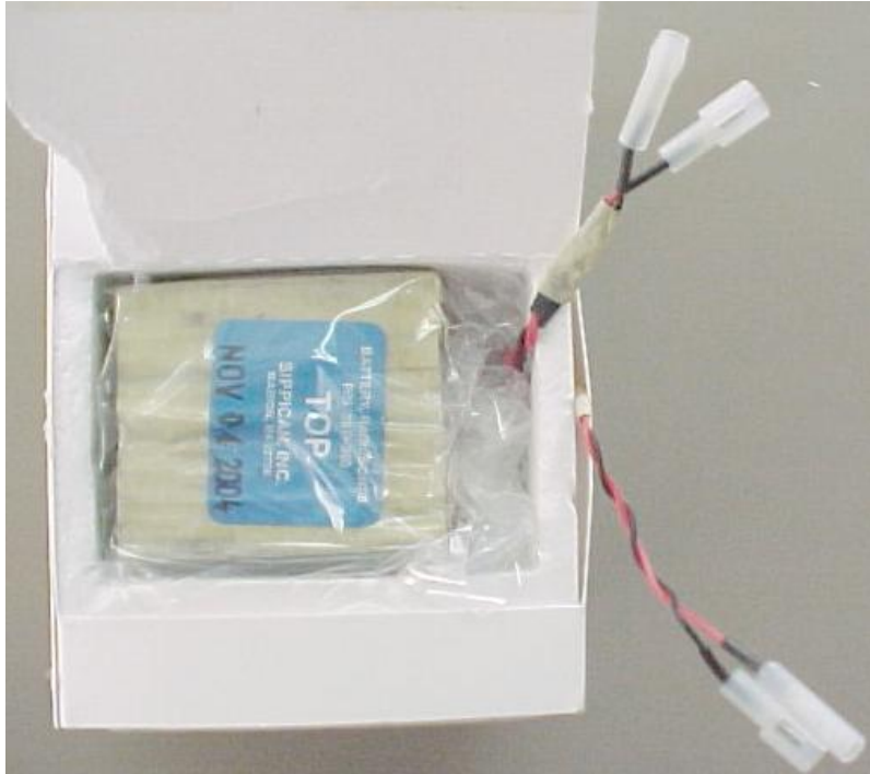
Figure N-12 – Twist Battery Wires
