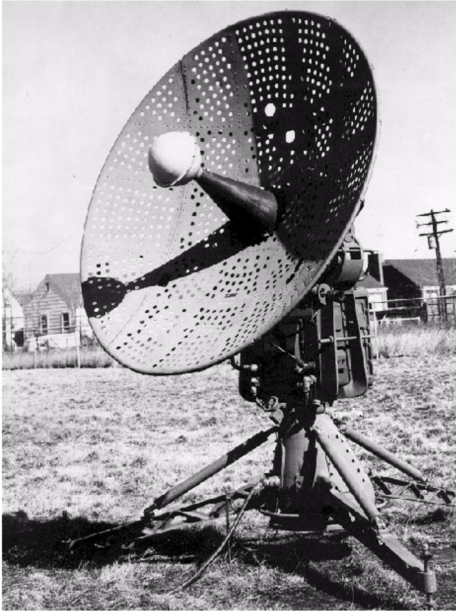
Figure B-3 - GMD Antenna/Pedestal Assembly (ART-1)
