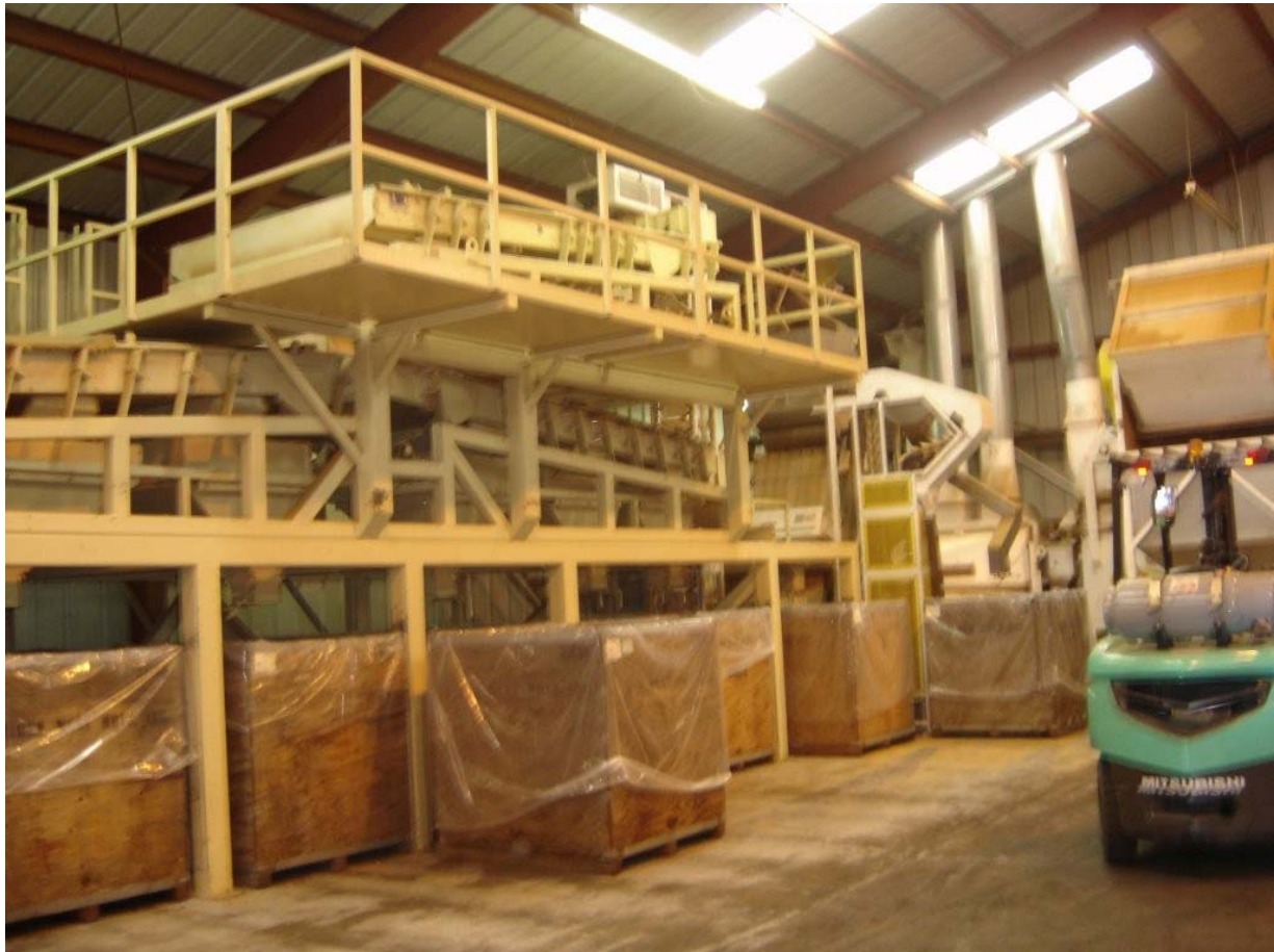
The large bins in this picture contain almonds at the intake stage of this plant's processing line. Nuts in this stage must be separated from those in other areas of the plant to eliminate the possibility of contamination.
