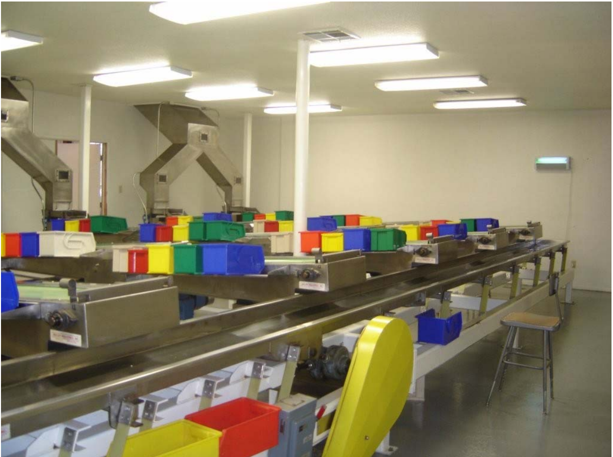
This room in an almond processing facility exemplifies GMP. Walls, floors and equipment are all made of materials that are easily washed and sanitized. Also note the ample amount of lighting. Note the insect electrocutor on the wall.
