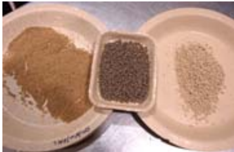
Plates made from biodegradable plastic hold powder (left) made from chicken feathers. This powder is processed into pellets (center and right) for use by manufacturers.
