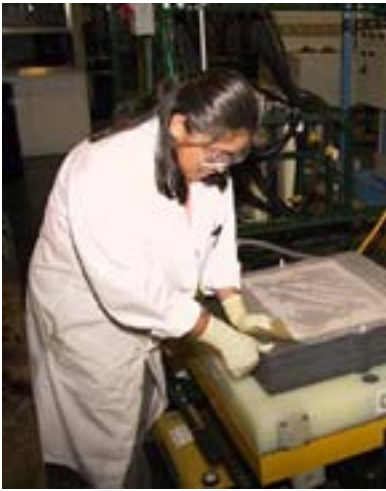
Chemical Engineer, Paula Moon inspects the EDI wafer stack.
