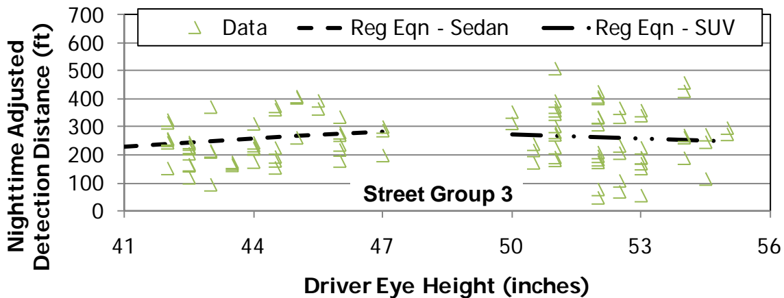
Figure 60. Graph. Nighttime adjusted detection distance by vehicle type and driver eye height for street group 3 at study sites.
