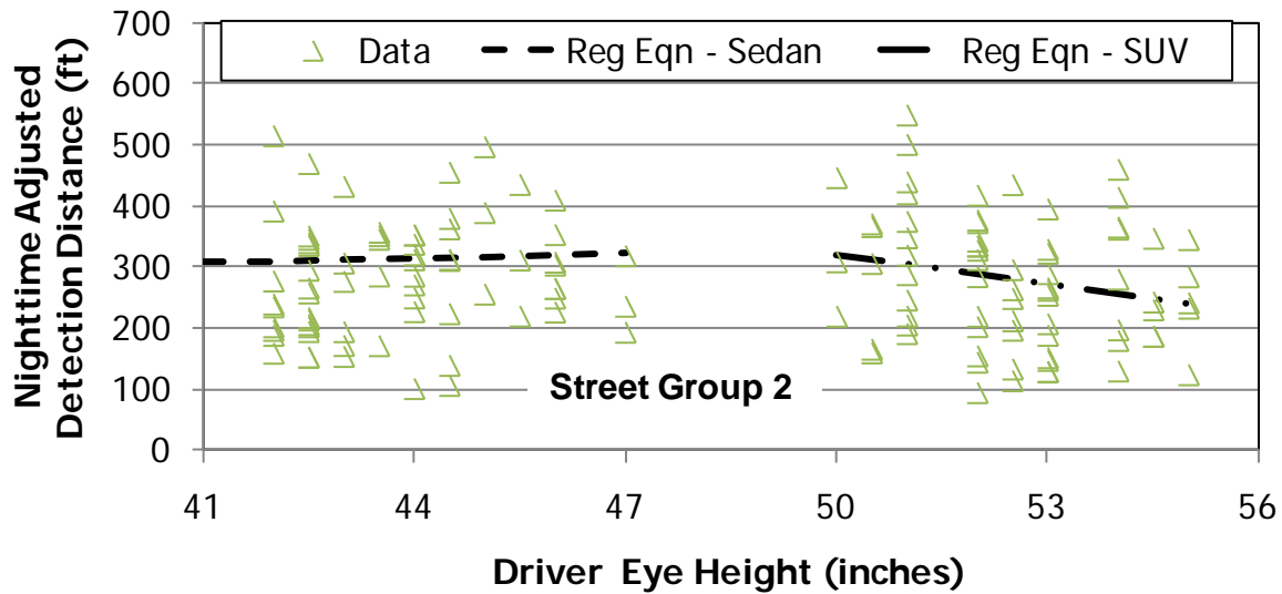
Figure 59. Graph. Nighttime adjusted detection distance by vehicle type and driver eye height for street group 2 at study sites.
