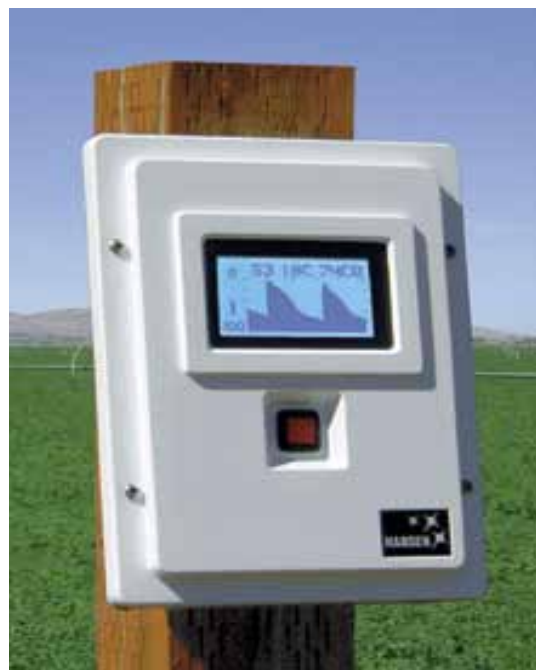
Figure 4. Sample Soil Moisture Data Logger with graphing
