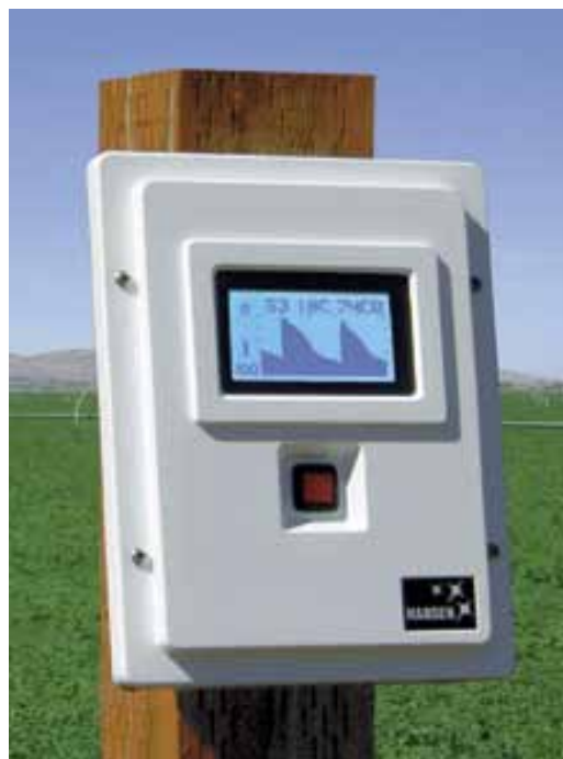
Figure 16. Soil Moisture data recorder with graphing
