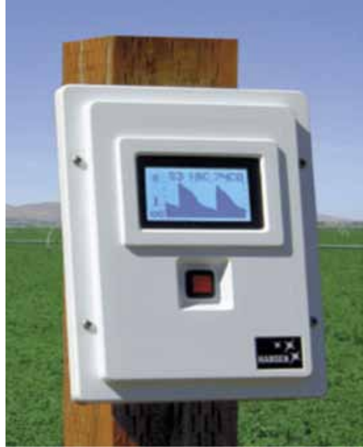
Figure 11. Soil moisture data recorder with graphing
