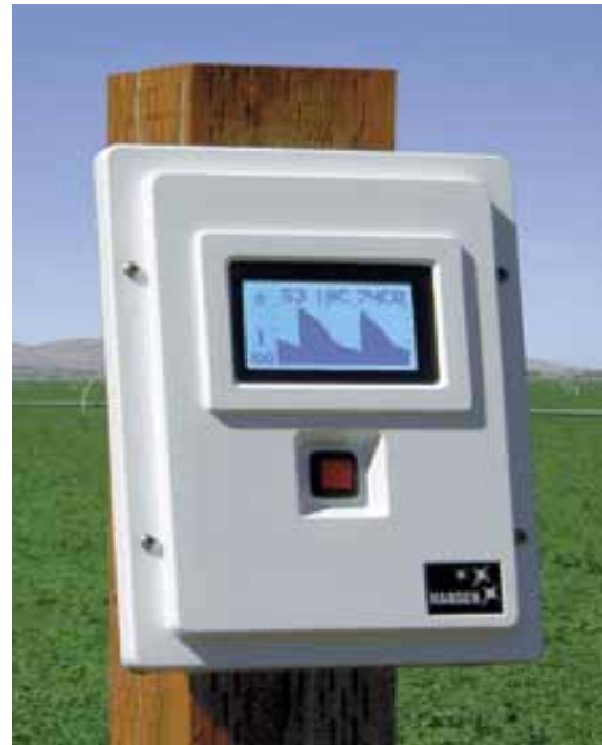
Figure 4. Sample Soil Moisture Data Logger with graphing
