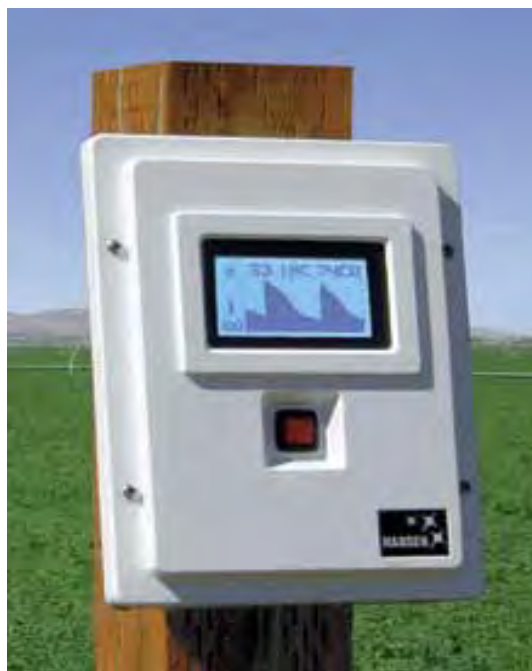
Figure 10. Sample Soil Moisture Data Logger with graph
