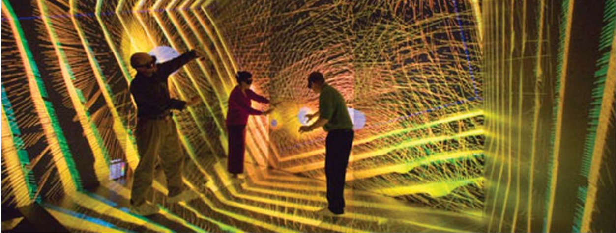
The CAVE Facility allows scientists and engineers to interact with full room 3D simulations and models.
