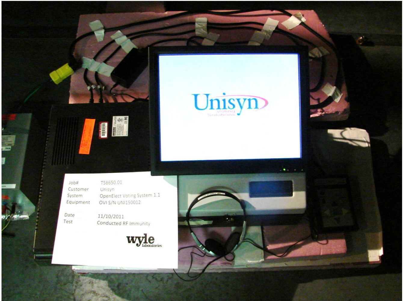
Photograph No. 9 OVI S/N UNI150022 Conducted RF Immunity -1
