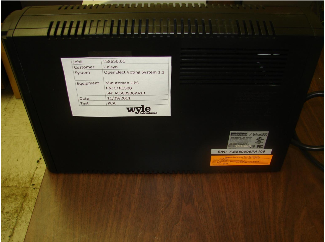
Photograph No. 40 OpenElect Voting System 1.1 Minuteman UPS P: ETR1600; SN: AES80906PA10
