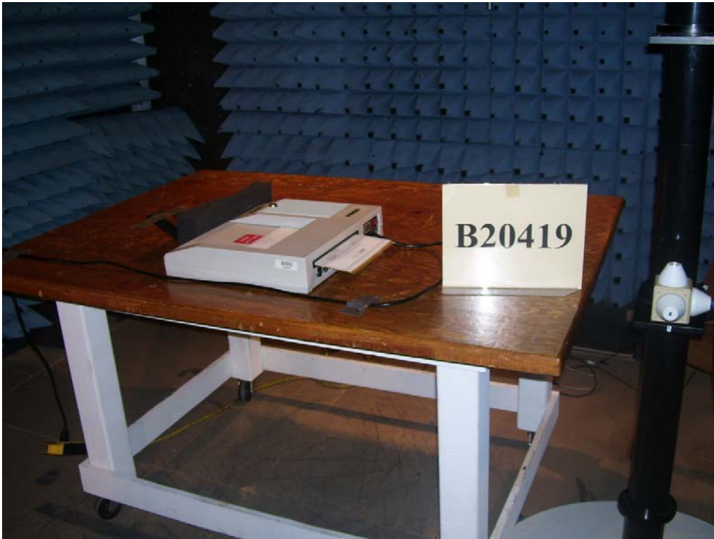
Figure A2. Radiated RF Immunity Test Setup – Right Side.
