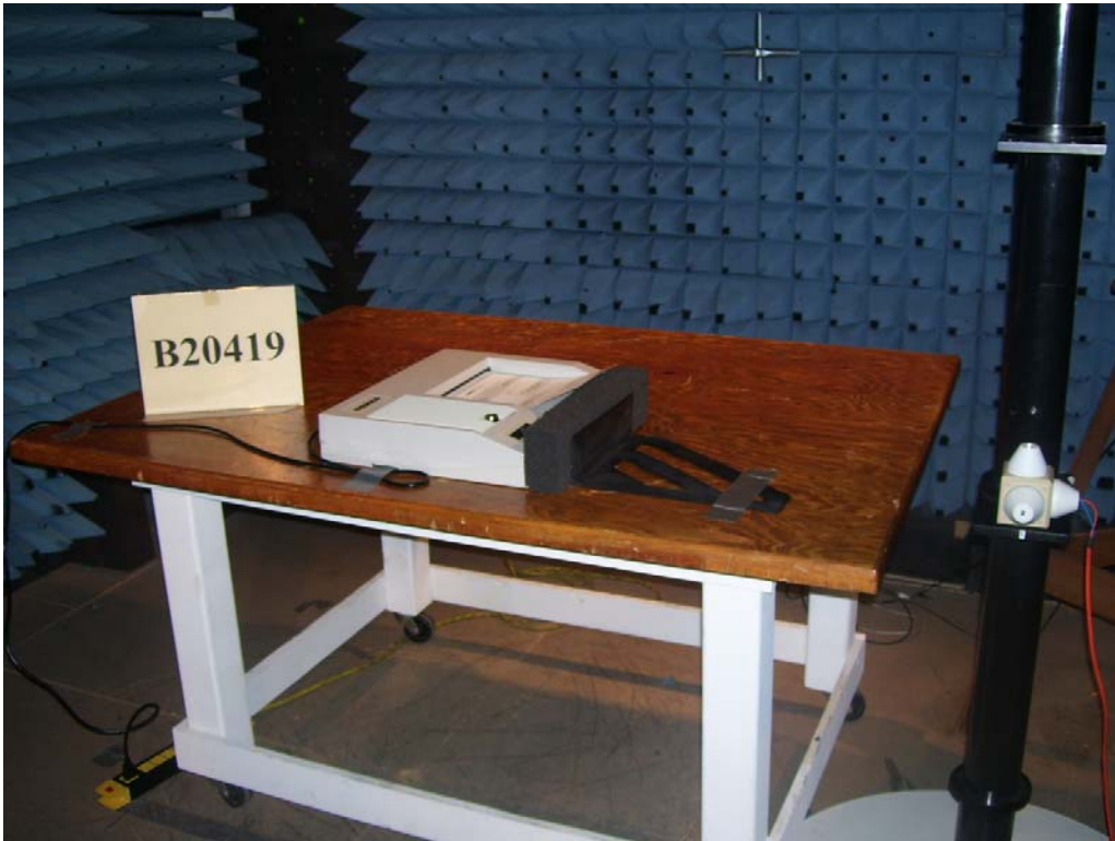
Figure A4. Radiated RF Immunity Test Setup – Left Side.
