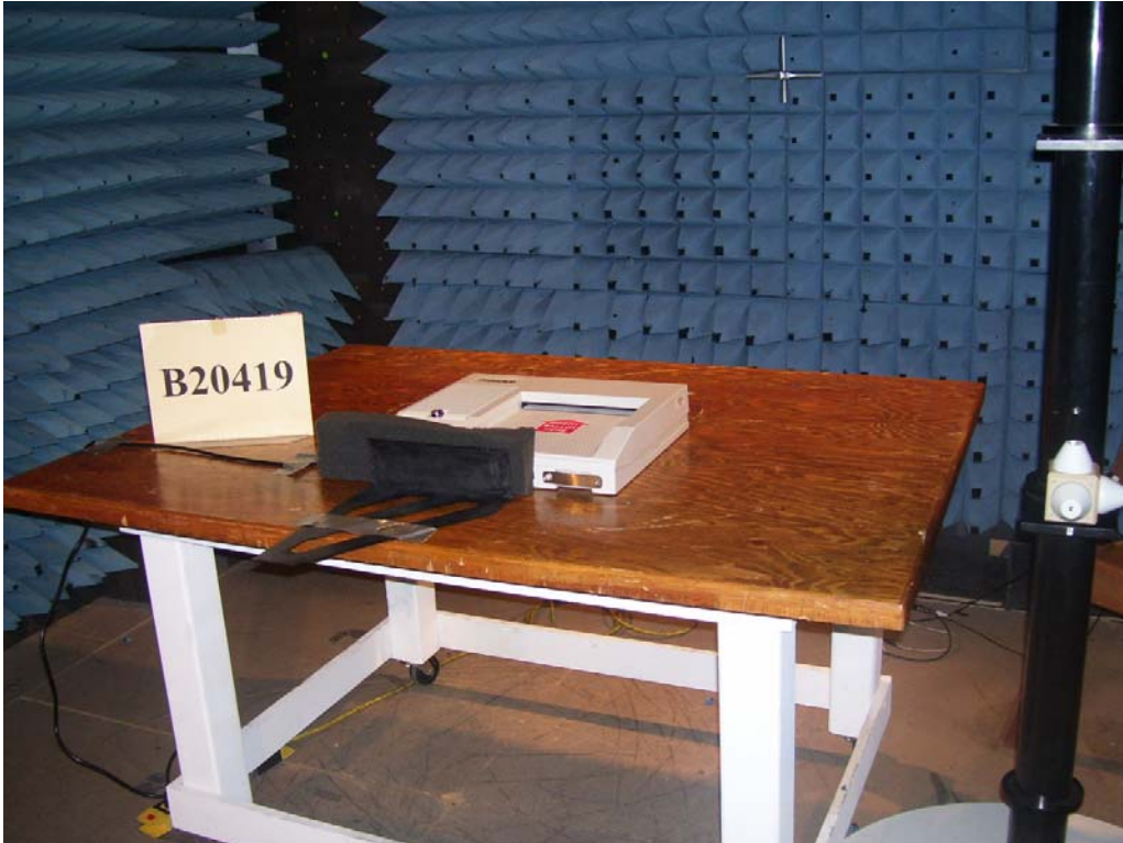
Figure A1. Radiated RF Immunity Test Setup – Front Side.
