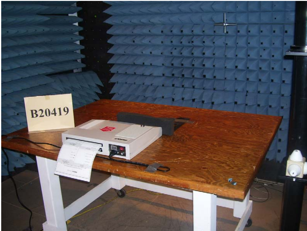
Figure A3. Radiated RF Immunity Test Setup – Back Side.
