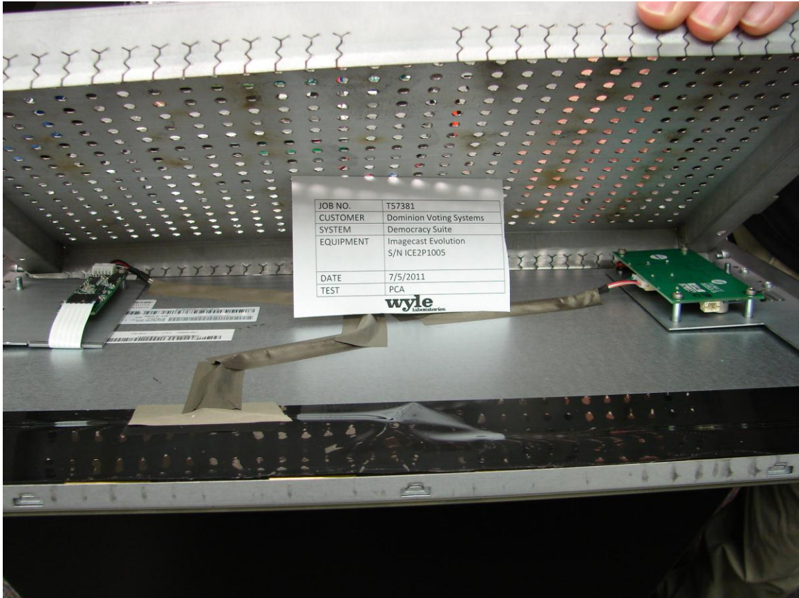
ICE internal shielding
