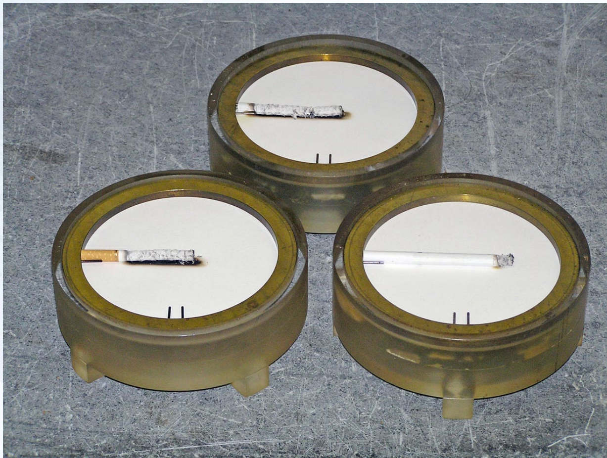
Examples of results of the Standard Test Method for Measuring the Ignition Strength of Cigarettes (ASTM E2187) are shown. Non-filter (top) and filter (left) cigarettes “failed,” having burned the full length in the test. The cigarette that extinguished before burning its full length (right) passed. The test calls for performing 40 such determinations for each cigarette and reporting the number of full-length burns. Cigarettes are positioned on the standard ASTM E2187 test substrate. Credit: NIST
