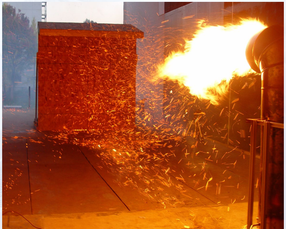
NIST's Firebrand Generator generates burning embers (or firebrands) that are major sources of ignition of house fires during blazes at the wildland-urban interface (WUI). Photo credit: NIST
