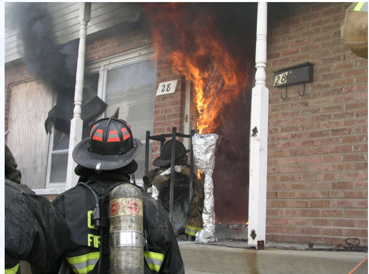
Flames from a living-room pour out the front door of a townhouse in NIST tests that studied conditions that can result in the failure of the facepiece lens of the self-contained breathing apparatus worn by firefighters. Facepieces were outfitted with devices to record temperatures and then mounted on a headform test stand placed outside doorway. The foil-wrapped equipment to the right of test set-up measured thermal heat flux. Credit: NIST
