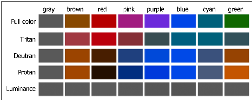
Figure 9. The colors from Figure 8 as seen by dichromats (Vischeck simulation), plus their luminance (all the same). Only blue and brown remain distinct for all forms of CVD.
