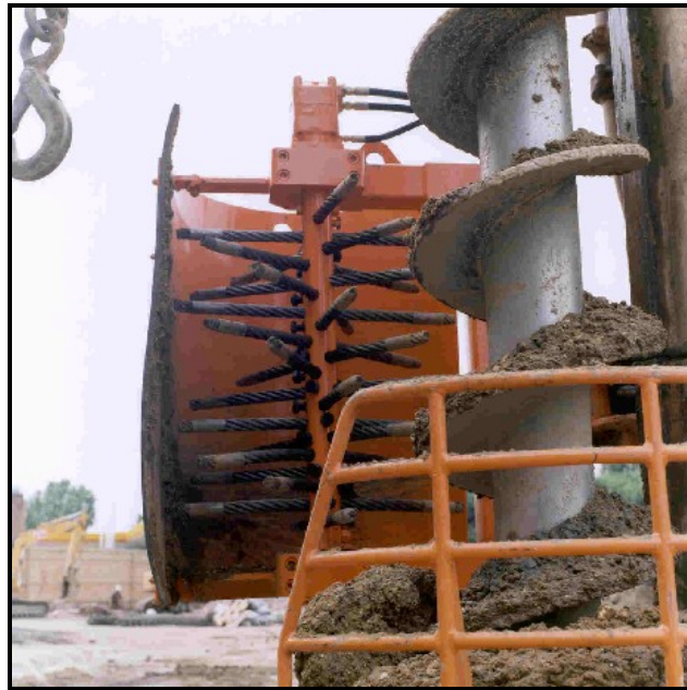
Figure 4.8: Auger for Use in Clay, with Auger Cleaner Attachment
