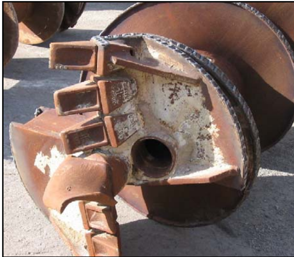
Figure 2.7: Hole at Base of Auger for Concrete
