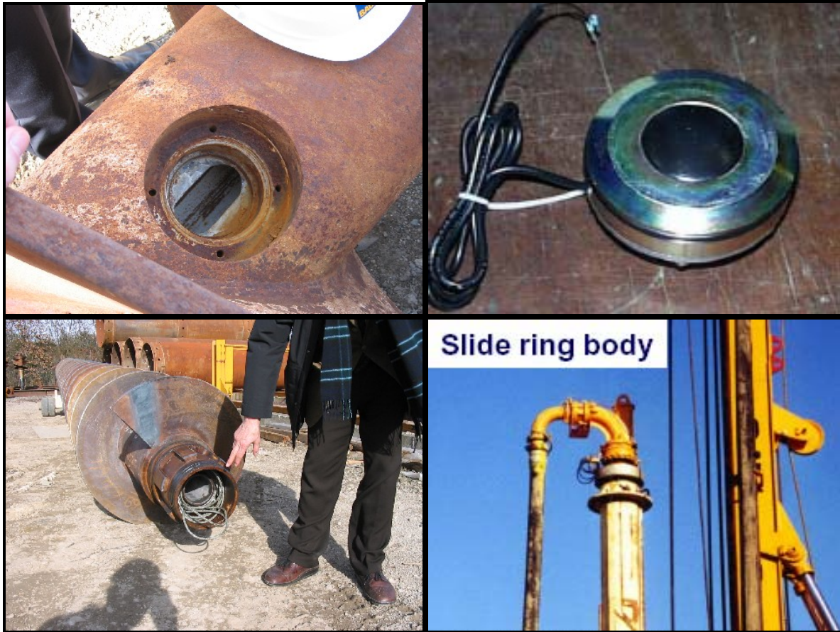
Figure 4.21: Sensor for Concrete Pressure at Auger Tip
