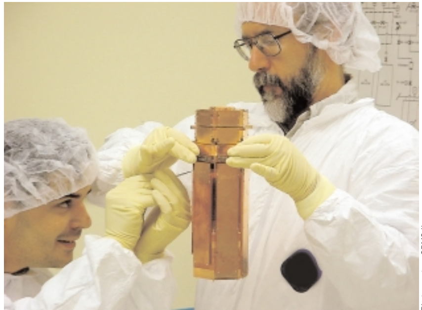
Project manager Dan Bauer from Fermilab holds one tower of detectors as Vuk Mandic from UC Berkeley examines them. Each tower of detectors contains 1 kilogram of germanium for detecting dark matter and 200 grams of silicon to distinguish WIMPs from neutrons. Thin layers of silicon, aluminum, and tungsten covering the detector surfaces measure both the heat and charge released when a particle interacts inside.
