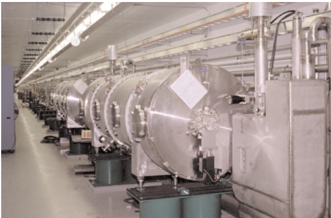
The first cryogenic tanks with superconducting RF cavities, built by Jefferson National Laboratory, are now in their final location within the SNS Linac.
