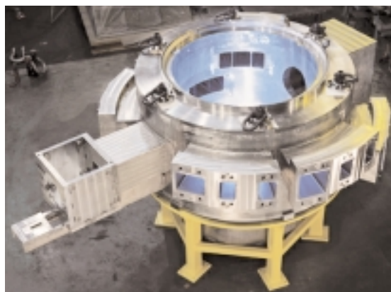
A 1-GeV proton beam will hit a mercury target at the center of this vessel, creating neutrons flying in all directions. Twenty-four “windows” allow neutrons to travel to experimental set-ups surrounding the vessel.
