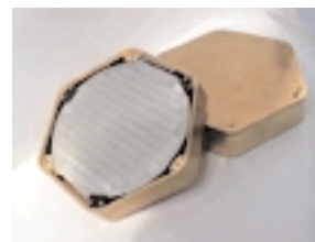
Individual silicon detectors like these operate in stacks at close to absolute zero.
