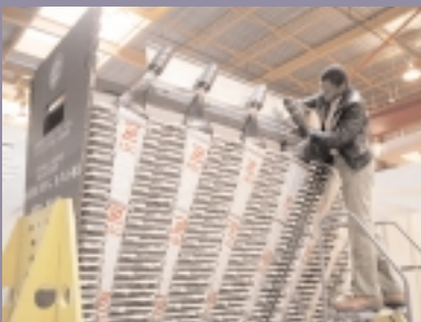
An employee installs a photo multiplier tube in a calorimeter unit for the CDF detector.
