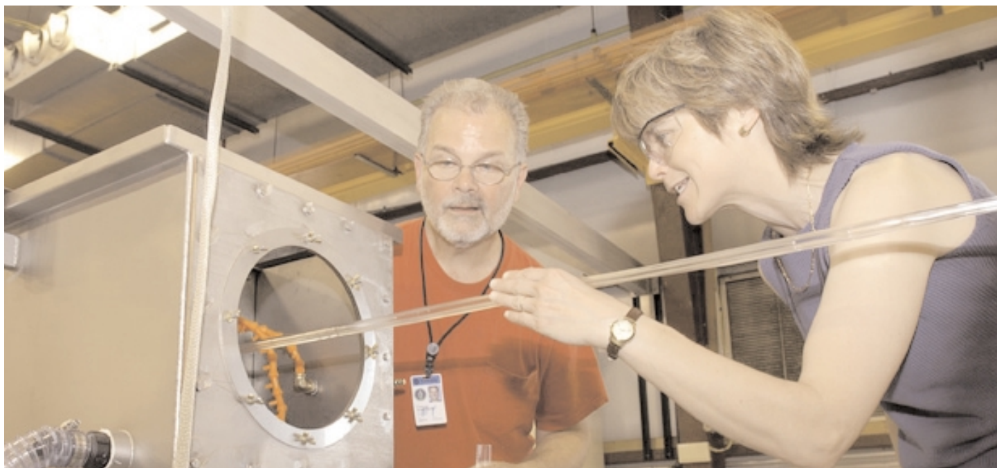
Chuck Serritella and Anna Pla-Dalmau get a feel for scintillating plastic emerging from the extruder line.
