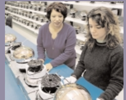
Sabina Aponte (left) and physicist Fernanda Garcia prepare photomultiplier tubes for MiniBooNE.
