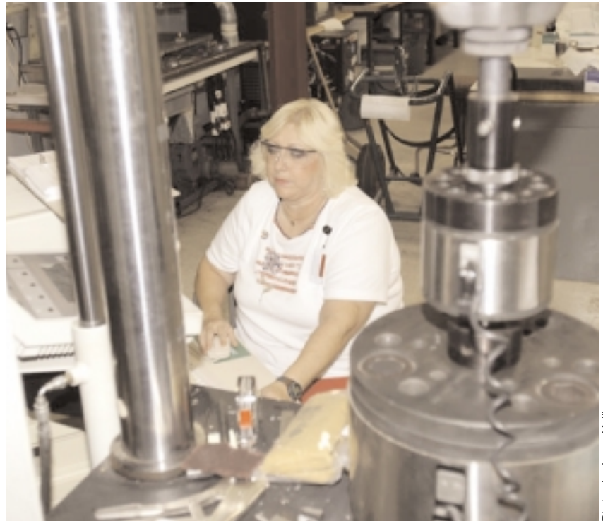
Hicks testing the tensile strength of an experiment's component using the Instron—an universal mechanical strength-testing machine.
