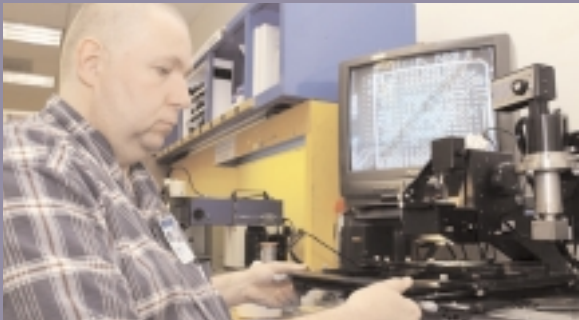
Bill Barker inspects Ball Grid Array at Feynman Computing Center.
