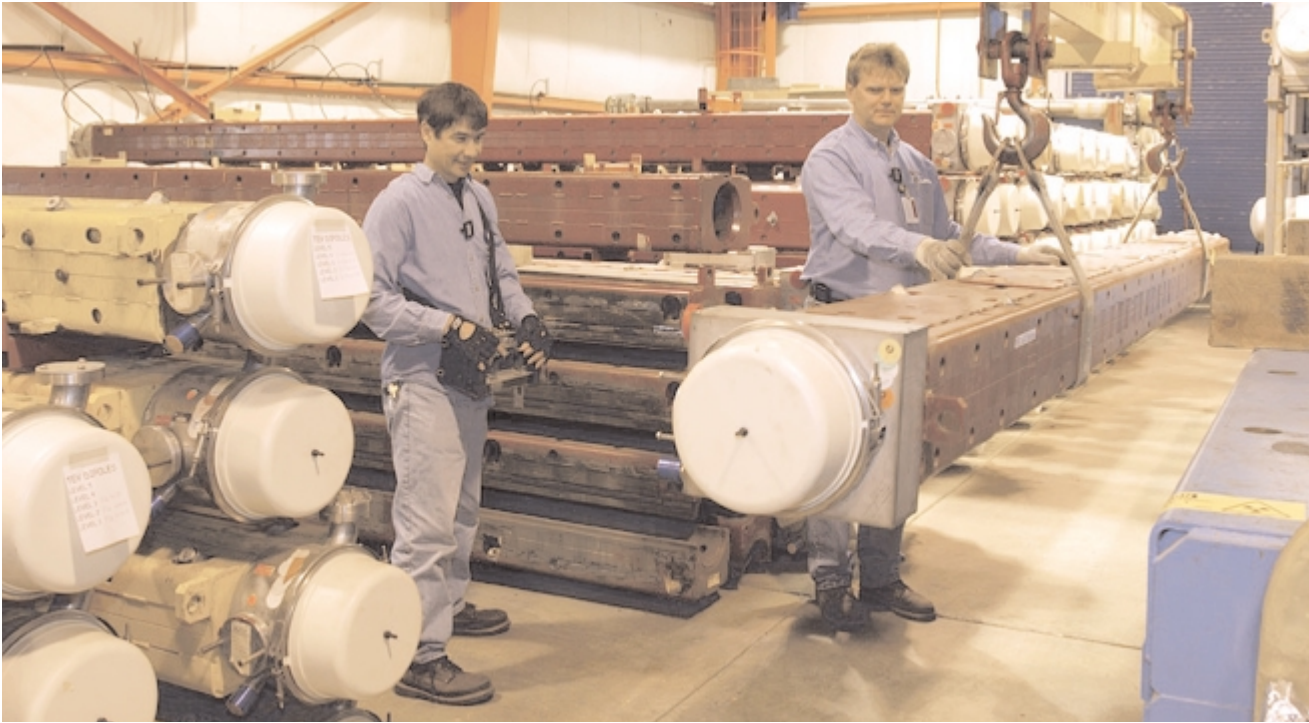
Doug Kelley (left) and Cliff Besch remove a spare Tevatron dipole magnet by overhead crane, in the Magnet Storage Building. Material Control keeps track of more than 1,000 backup magnets.
