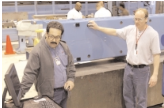
Oscar Lira (left) and Ted Beale use the Laser Tracker to compare the straightness of a B2 dipole magnet in various orientations, ensuring tight tolerances for NuMI’s primary proton beam.
