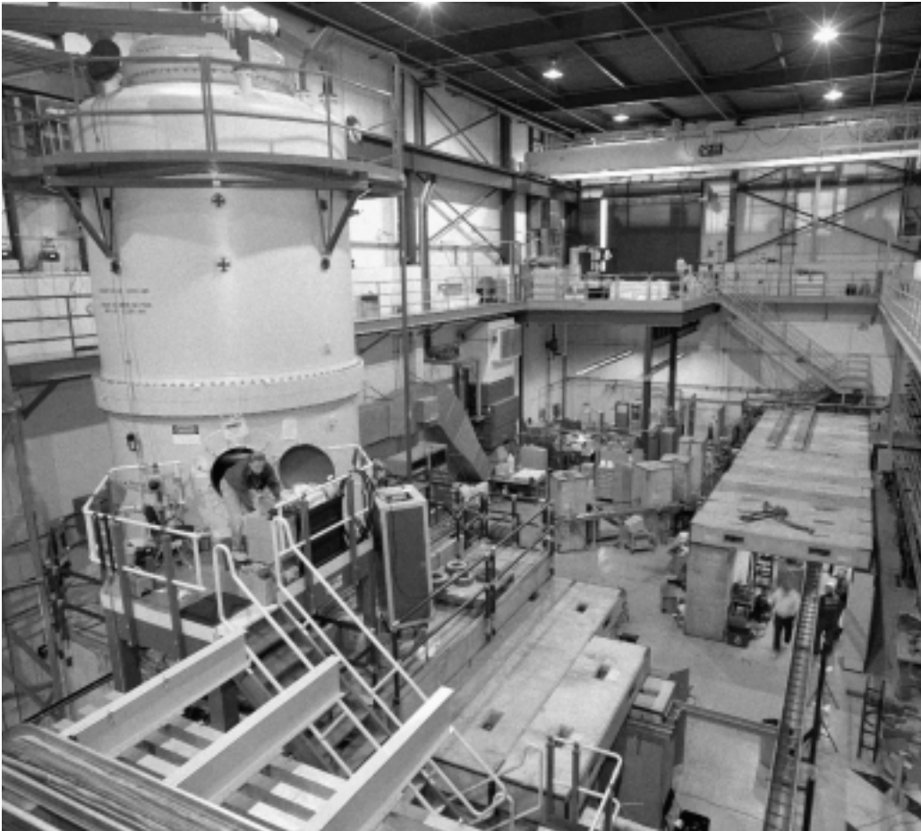
The research facility for electron cooling project includes a 25-foot-high Pelletron accelerator (left), which produces a continuous high-energy electron current with the highest beam power in the world. Scientists plan to extract the beam, send it through a 60-foot-long cooling section (right, under construction) and return the electrons to the Pelletron for recirculation.
