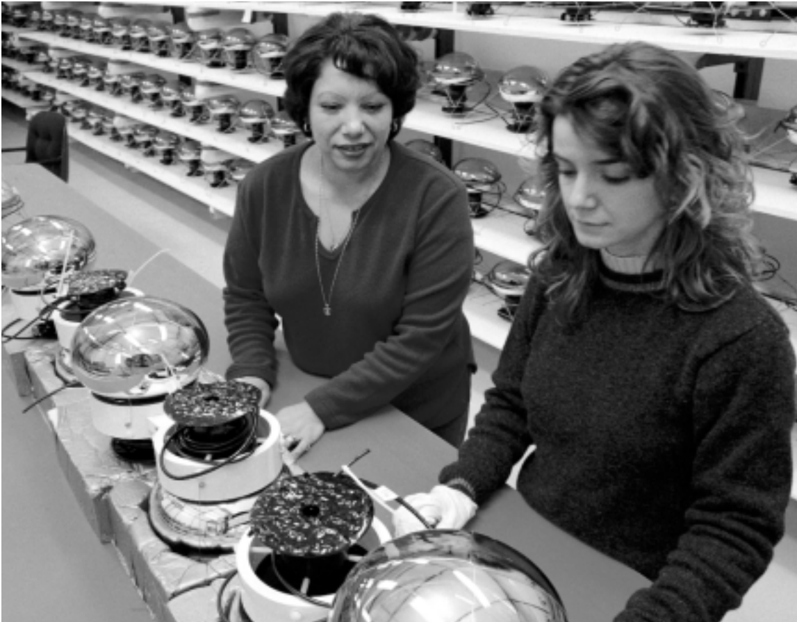
Fernanda G. Garcia (right) and Sabina Aponte prepare photomultipliers which are provided to the installation crew on demand.
