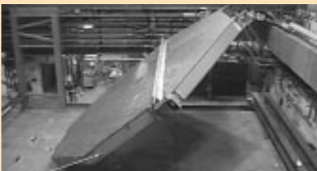
A layer of steel and scintillator is raised on a strongback, in a simulation of operations for assembling the MINOS detector.
