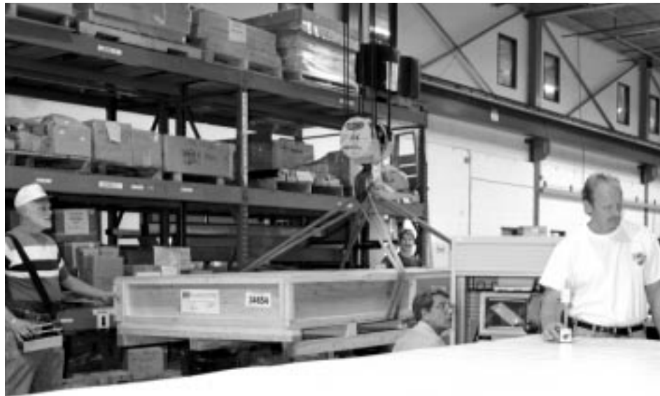
In the foreground, Ted Beale (right) and Steve Merkler use a laser system to measure the flatness of a CMS Endcap Muon Chamber panel. In the background, Gary VeZain (left) and Doug Kelley direct a slings carrying a crate of the panels.
