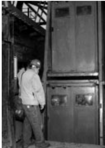
A 5,400-ton detector will be loaded, piece by piece, into this elevator, and carried down into the Soudan mine, 2,400 feet below ground.
