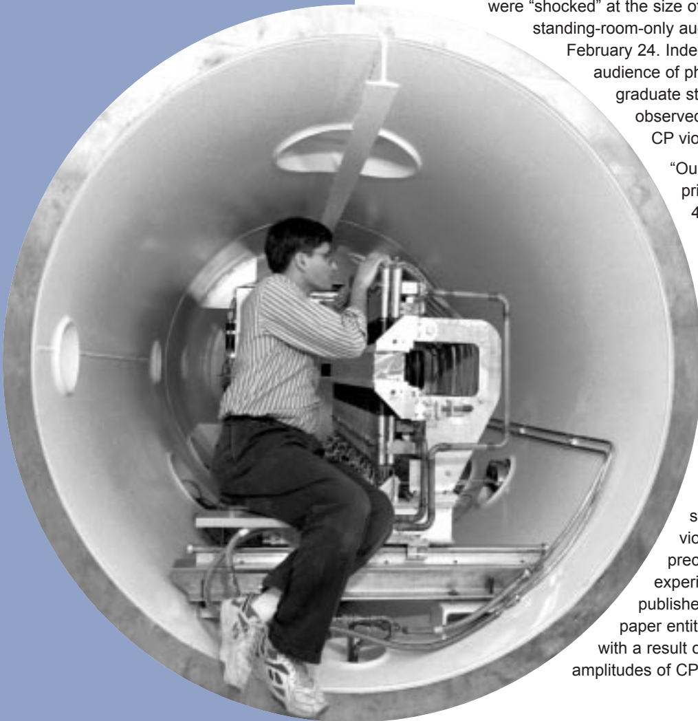
Amit Lath, from Rutgers University, checks the active scintillation counter regenerator inside the vacuum tank upstream of the KTeV detector.
