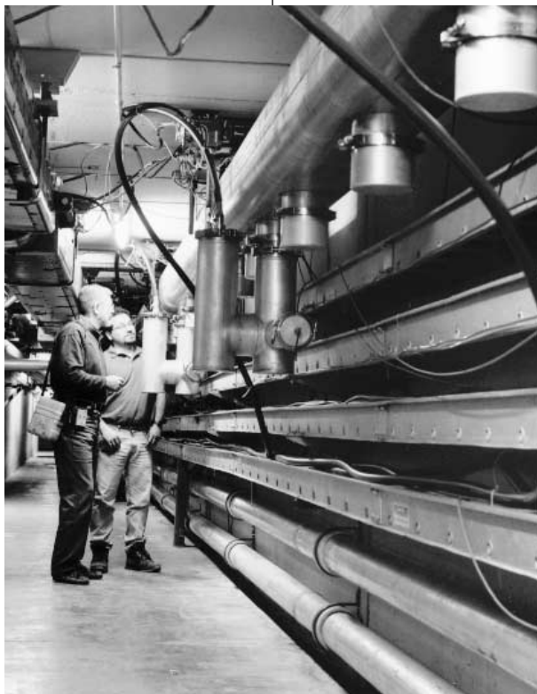
Craig Moore and Salah Chaurize examine septa in the Switchyard that split beam between meson and neutrino.
