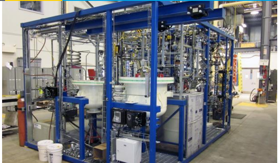
Gas Technology Institute's 50kg/d IH 2 pilot unit to be installed at GTI's main facility in Des Plaines, IL
