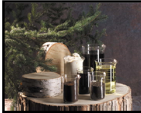
Mill residue feedstock and bio-oil and char products.
