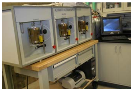
NREL's bench-scale catalyst microactivity test system.
