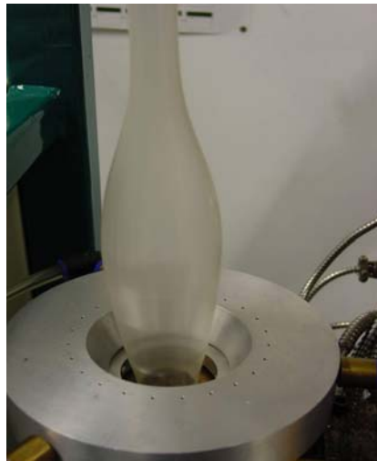
The first demonstration of film blowing with a PHA resin. Although there is much work still to be done to obtain a commercial process, this is a crucial first step.
