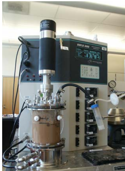
Lab fermentor for ethanol production research
