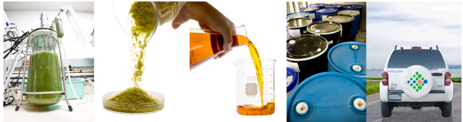
CAPTION: Left to right: (a) Laboratory scale fermentation of algae (b) Dried algal biomass (c) Purified algal oil (d) Thousands of gallons of algal oil have been produced in non-integrated tolling facilities. Solazyme algal oils have been refined to transportation fuels that meet industry specifications. (e) Solazyme’s biodiesel and renewable diesel have powered a light truck and three cars with unmodified diesel engines for thousands of miles on the open road (with blends ranging from B20 to B100).
