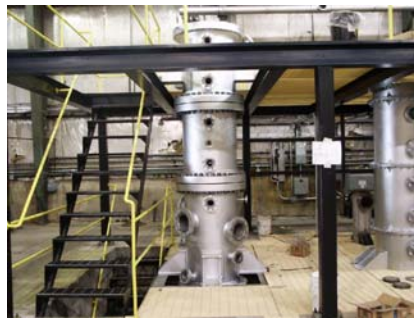
Fluidized bed black liquor gasification test system
