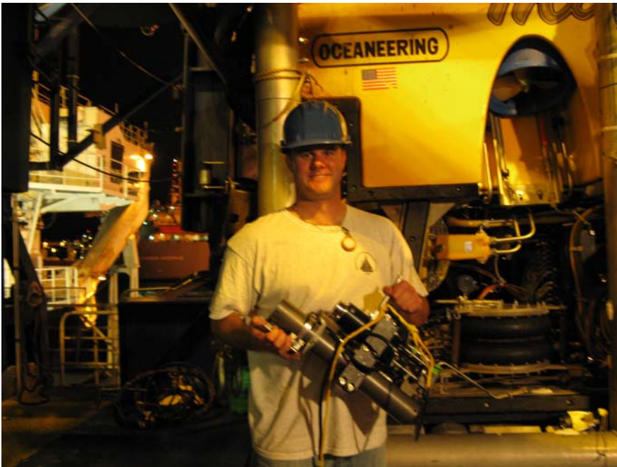
Fig. 8: Image of the IGT sampler prior to integration onto the Millennium 42 ROV on June 20-21, 2010.
