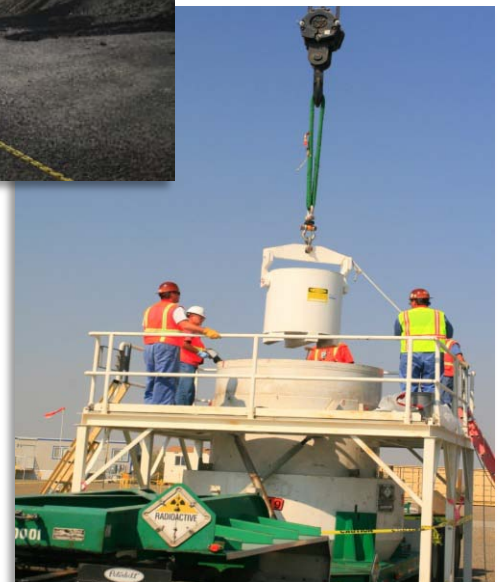
Off-loading Hopewell 7A Cask from 10-160B Shipping Cask
