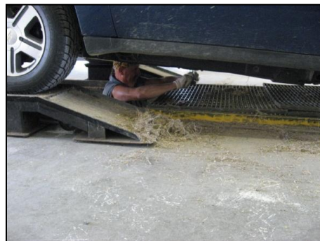
Weeds removed from the skid plate area of four-wheel drive vehicle
