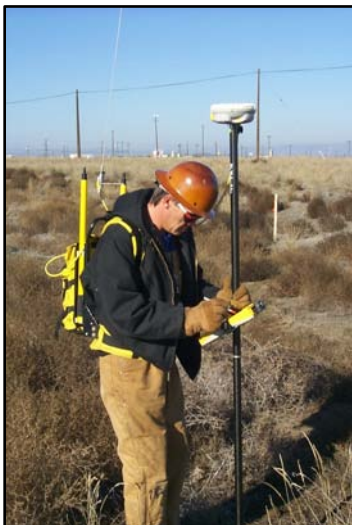
Field Sampling Survey using a Global Position System (GPS)
