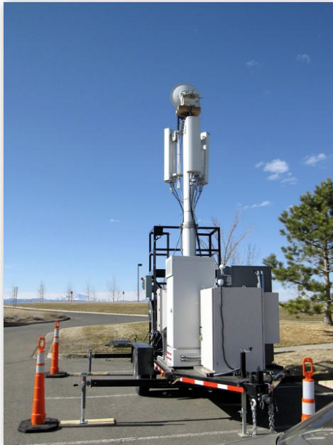
Figure 6.1: Mobile “Cell on Wheels,” an element of the Department of Commerce Public Safety Communications Research (PSCR) Public Safety Broadband Demonstration Network.
