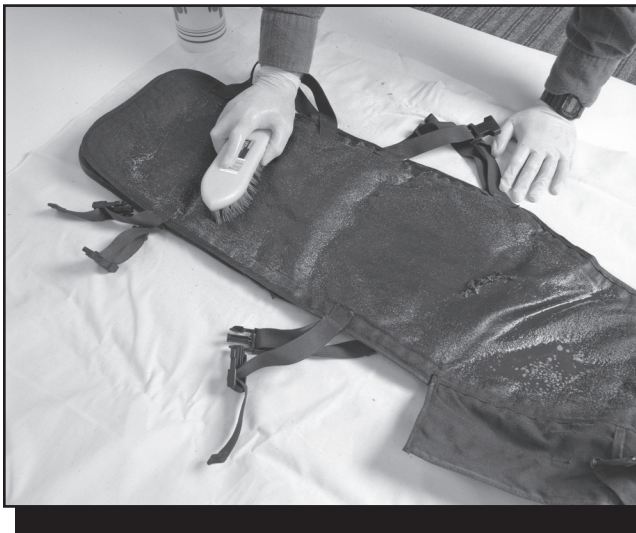
Figure 5—Clean lightly soiled chaps with a CitroSqueeze solution and a scrub brush.
