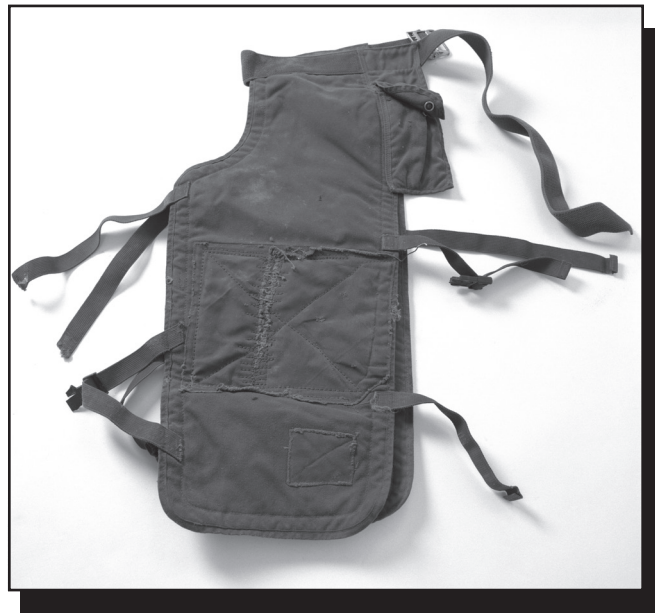
Figure 4—Retire chaps when they have been improperly repaired by stitching through the protective pad.
