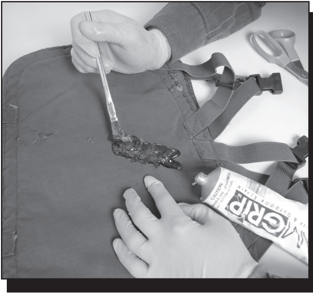
Figure 7—Spread Seam Grip over the entire hole.
