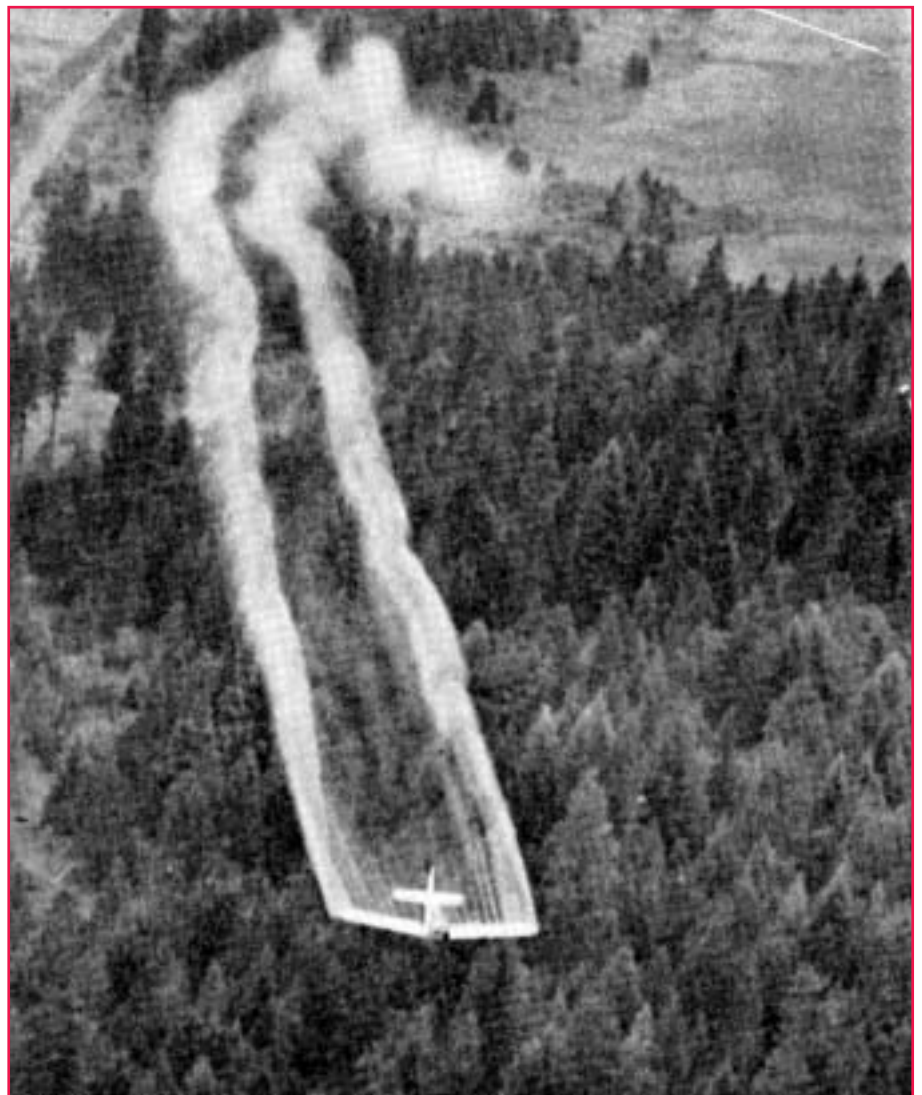
Figure 1 —Low-flying spray plane. Note funneling effect of spray trailing behind each wingtip. This is vortex turbulence.
