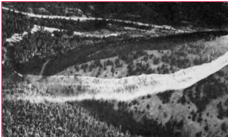
Figure 4—Wake from a DC-3 and pronounced vertical motion of the vortex.
