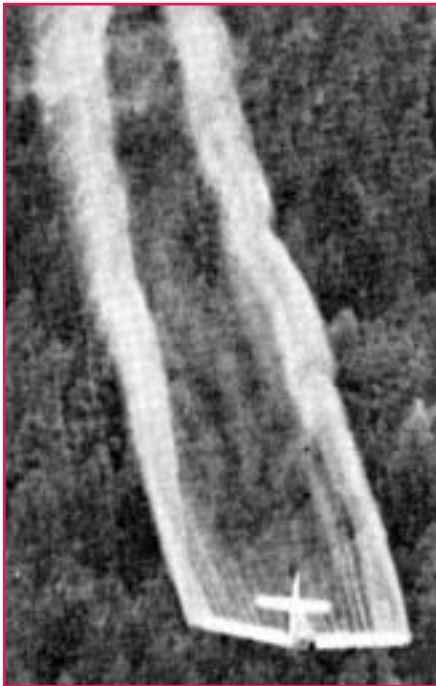
Figure 1 —Low-flying spray plane. Note funneling effect on spray trailing each wing.
