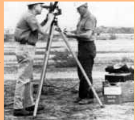
Fire behavior team takes a pilot balloon observation with theodolite to determine patterns of local winds aloft. Photo: USDA Forest Service.
