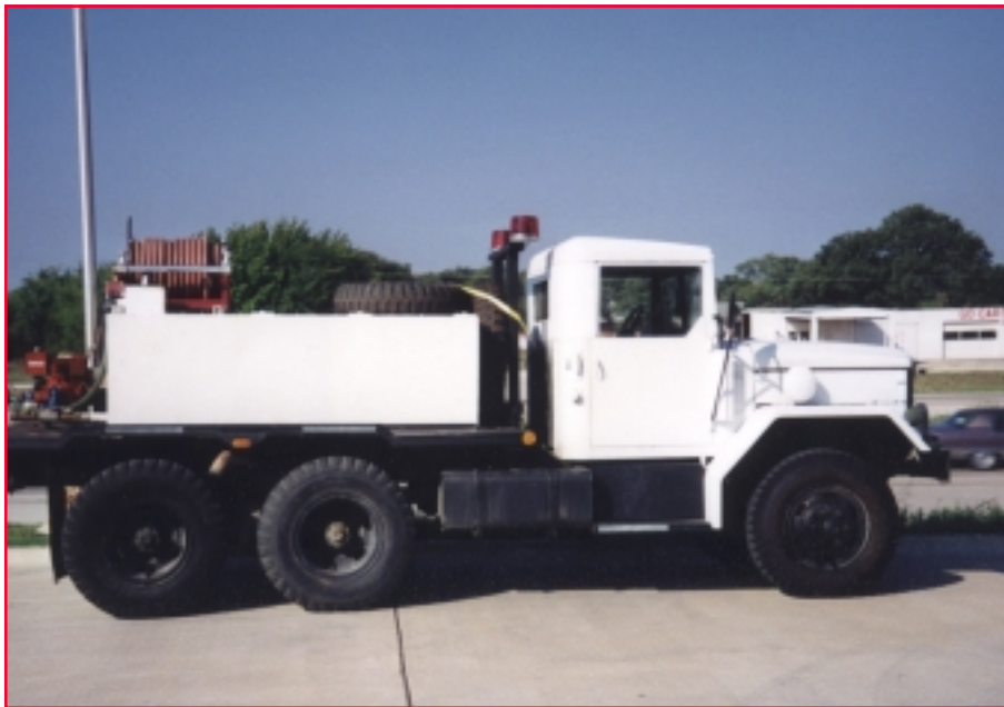
A private contractor donated this 750-gallon (2,839-L) pumper to the Texas Forest Service, which passed it on to the Lake Kickapoo Volunteer Fire Department through the Helping Hands Program. The program allows individuals and businesses to donate surplus fire equipment without worrying about liability costs. Photo: Texas Forest Service, 1998.
