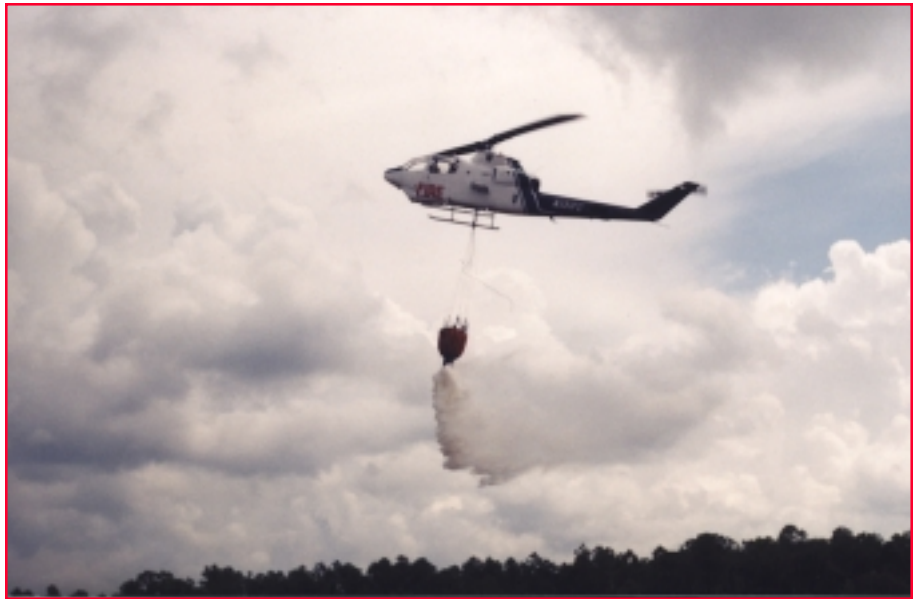
Skimming, usually no more than 200 feet (60 m) above the ground, a Fire Snake makes a training drop on Florida’s Blackwater River State Forest. Photo: Michael Kassinger, Milton, FL, 2001.
