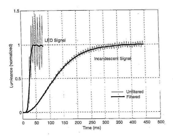
**Figure 1.** Rise times of a LED and an incandescent traffic signal measured in the field. The light line is the instantaneous signal luminance. The bold line is the trend in signal luminance smoothed through a filter.
