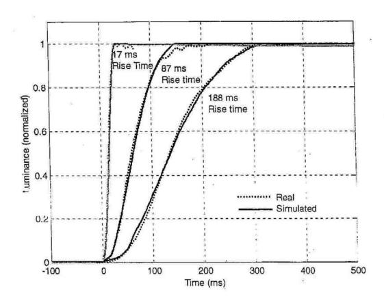
Figure 2. Smoothed rise time profiles for real LED and incandescent traffic signals measured in the field and the simulations of the same signals used in the experiment.
