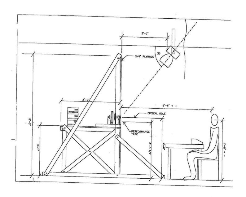
Figure 3. A schematic elevation of the apparatus
