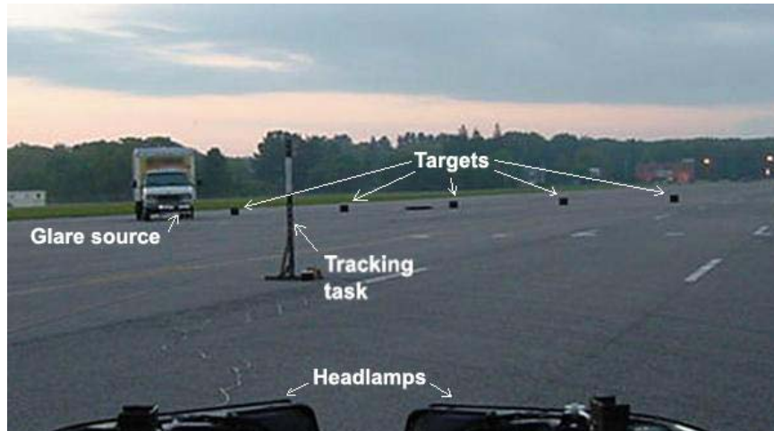
Figure II-5. Daytime view of the glare headlamps, small targets and tracking task, approximately from the subjects' viewing location.
