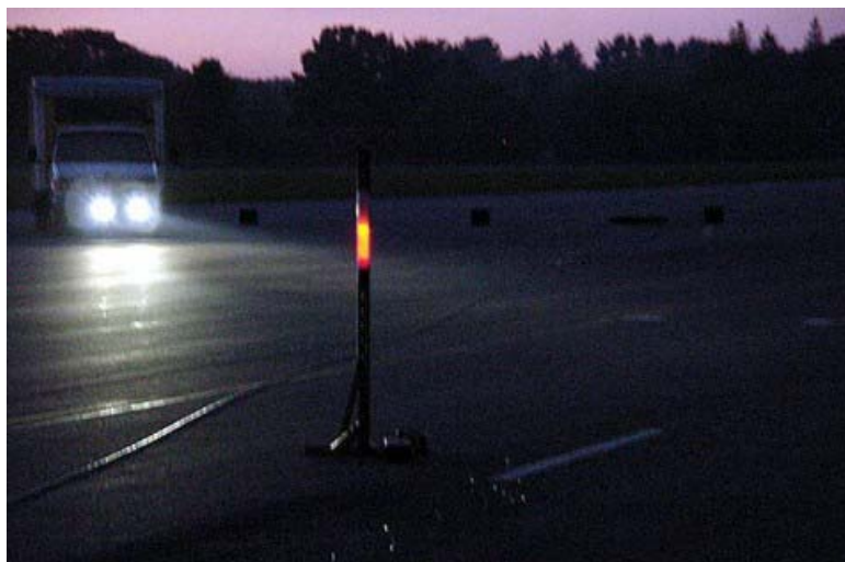
Figure II-6. View of glare headlamps, the three centermost targets and the tracking task as they appeared during experimental nighttime sessions.
