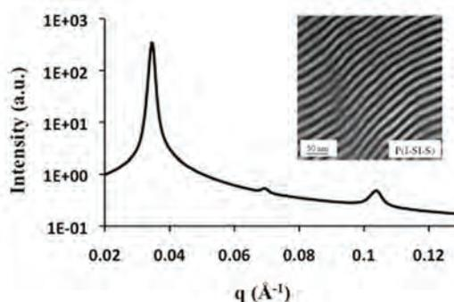
**Right bottom:** Synchrotron-SAXS data for a P(I-SI-S) tapered diblock copolymer. Specimens were annealed at 210 degrees C and then cooled to room temperature for data acquisition. The integral moduli values are characteristic of two-domain lamellae. The inset shows a transmission electron microscopy image of a P(I-SI-S) specimen. The sample is stained by OsO<sub>4</sub> vapor to enhance contrast.
