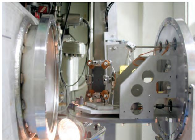
The X17A monochromator in the X17 front end, shown when rolled out of the chamber
