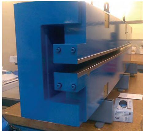
NSLS-II storage ring magnets — a total of 826 — include quadrupoles (**left**) and dipoles (**right**). The magnets are being built by vendors in six countries: China, Denmark, New Zealand, Russia, the United Kingdom, and the United States.
