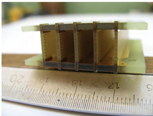
A miniature four-channel ionization chamber that was developed at NSLS
