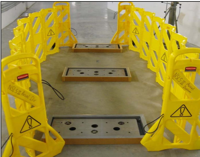
Figure 5. Multipole girder plates mounted on the floor.
