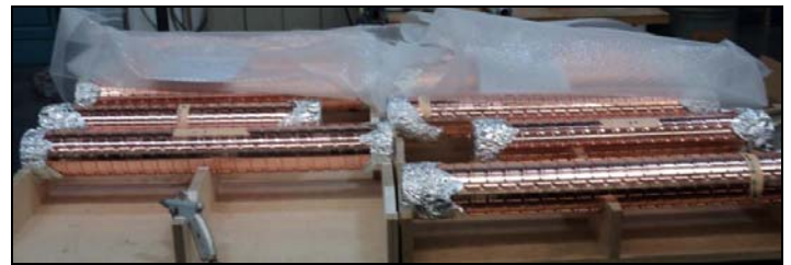
Figure 1. Accelerating structures of the NSLS-II linac. To complete the sections, cooling pipes will be brazed to the surface before final frequency tuning.
