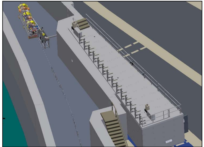
Figure 3. Optical diagnostic beamline and measurement hutch.
