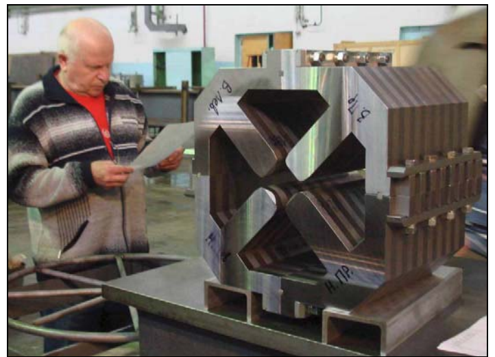
Figure 2. Completed yoke for a booster quadrupole magnet.
