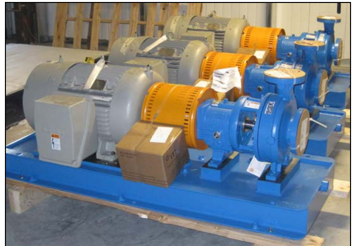
Figure 5. Water pumps for NSLS-II deionized water systems.
