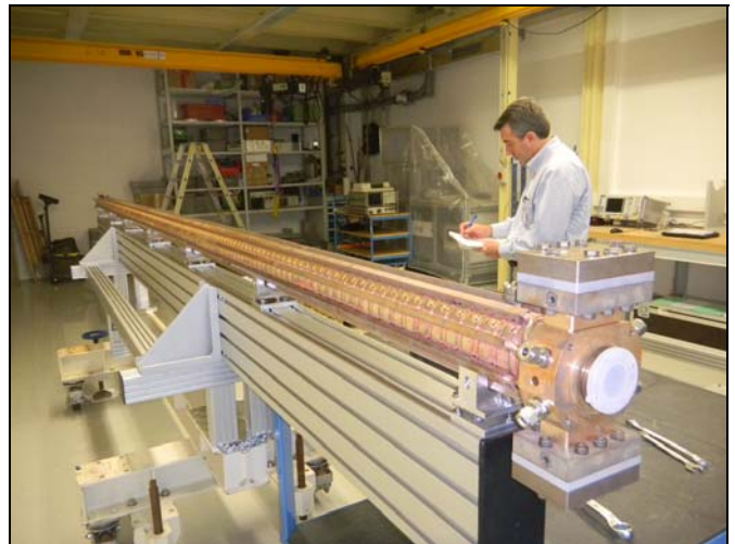
Figure 2. Final check on the 200 MeV linac accelerating structures.
