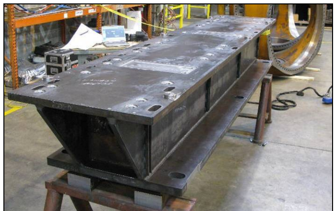
Figure 2. First article of the girder at the factory before painting and shipping.
